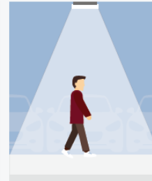
Light to full on (Occupant in full range)
